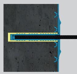
Accessories and Appurtenances (e.g. ladders, pipes, etc.) require proper mounting in concrete structures which are lined with concrete protective liner or HYDRO<sup>CLICK</sup>.
